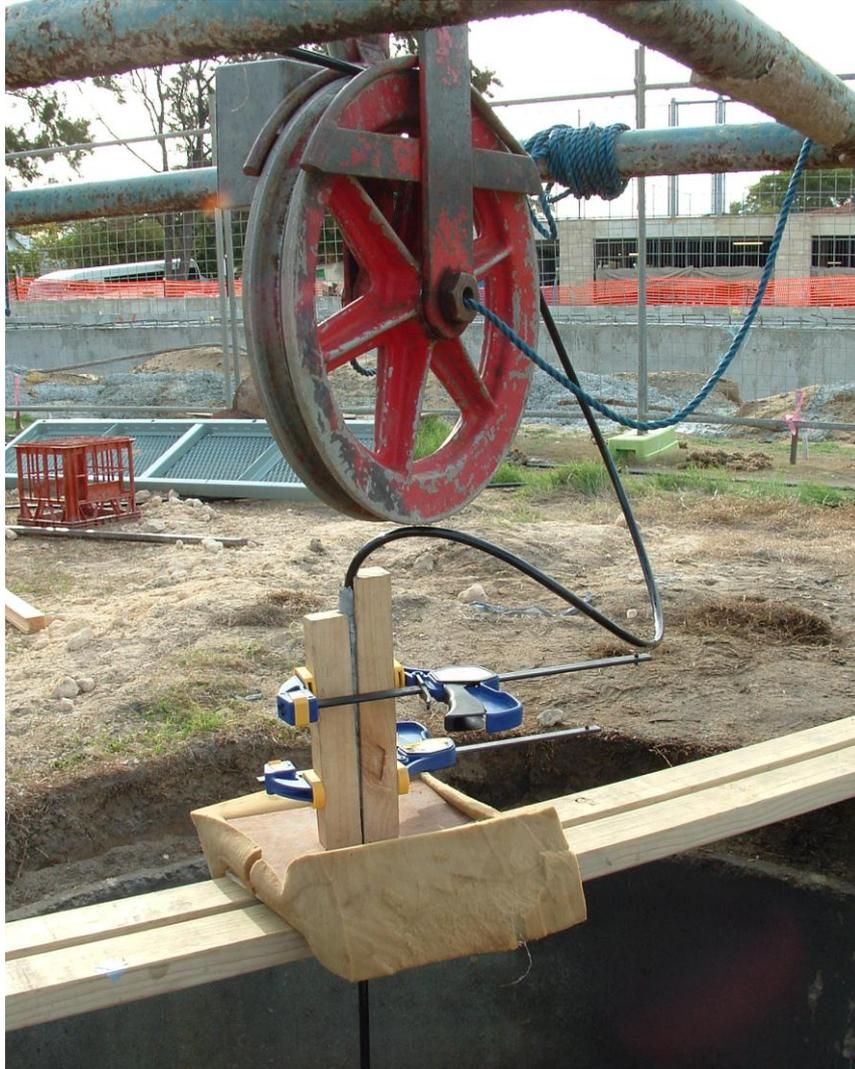
**Figure 4-2. Isolation of the hydrophone string from the sheave wheel by clamping the string and suspending it upon a plywood / foam sandwich. The sandwich board would normally rest directly on the borehole collar.**
