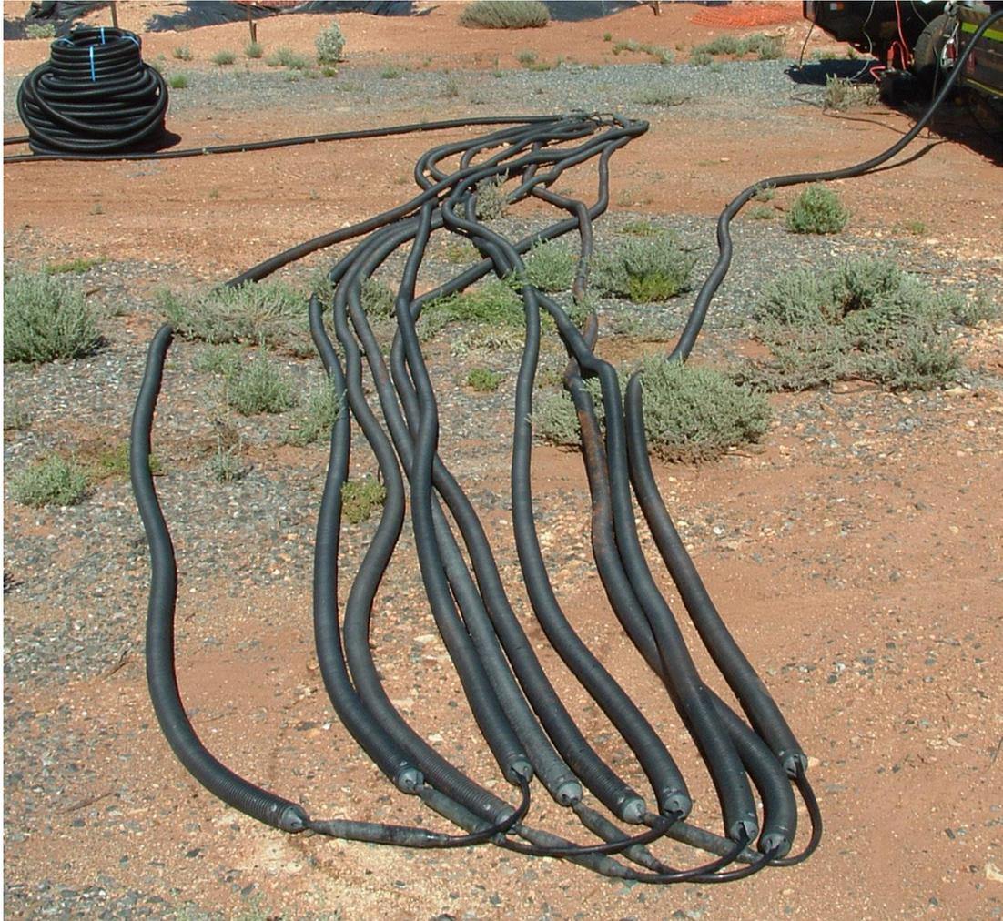
**Figure 4-12. 50 mm corrugated baffles installed on the lower 12 channels of the hydrophone string.**
