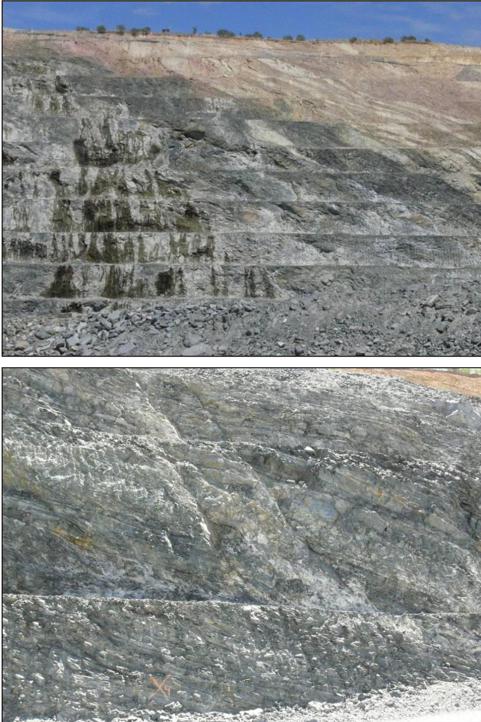
**Figure 3-15. Photographs of Ranger 3 pit. For scale, each bench is approximately 10 m high. Photo A shows the dominant 30° easterly dip of the Ranger deposit. Photo B demonstrates the structural complexity, high angle thrust and relaxation faults and scale of features.**
